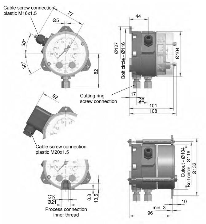
Illustration 6: Pressure chamber in aluminium (IP55)
