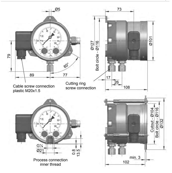
Illustration 7: Pressure chamber in aluminium (IP65)
