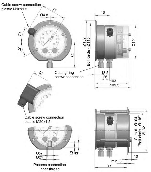
Illustration 8: Pressure chamber in VA (IP55)
