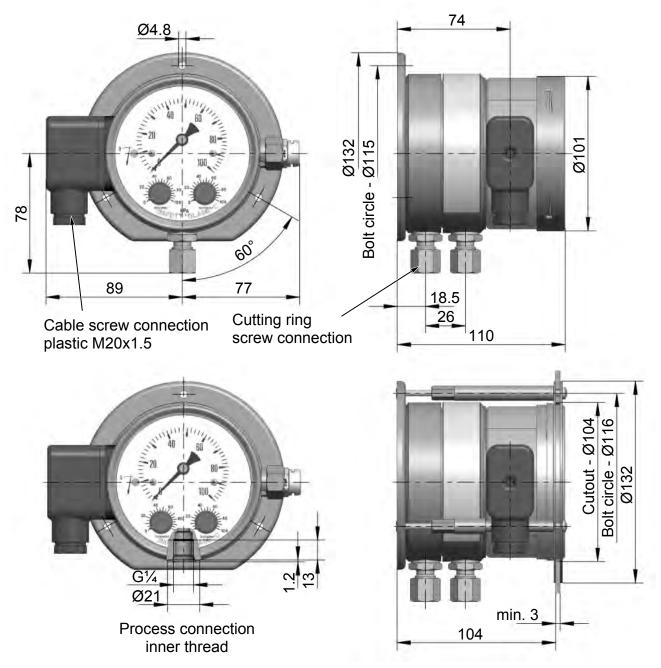
Illustration 9: Pressure chamber in VA (IP65)
