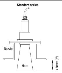
The horn must protrude at least 50mm (2") into the vessel
