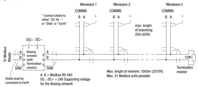
Additional use of 4-20mA output and Relay should be wired in a sparate cable, not mixed with the Modbus network.
