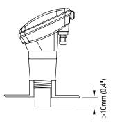
The face (membran) of transducer must extend at least 10mm (0.4") into the vessel. See dimension on page G8.
