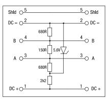
Biasing network PK6 with integrated Terminal resistor
