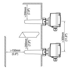
Observe mounting angle to ensure, that the active tip of the probe has enough distance to the metal silo wall
